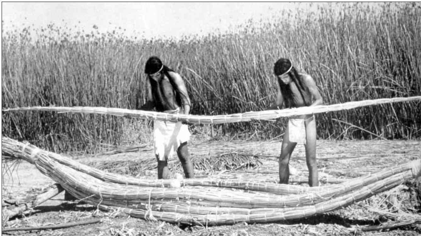
Boats were made with bundles of tules, they often leaked but did not sink. Boats were used for transportation to trade with Indians from other villages. Photo: Bowers Museum Collection
